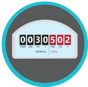
The water meter above is reading 30,502L
