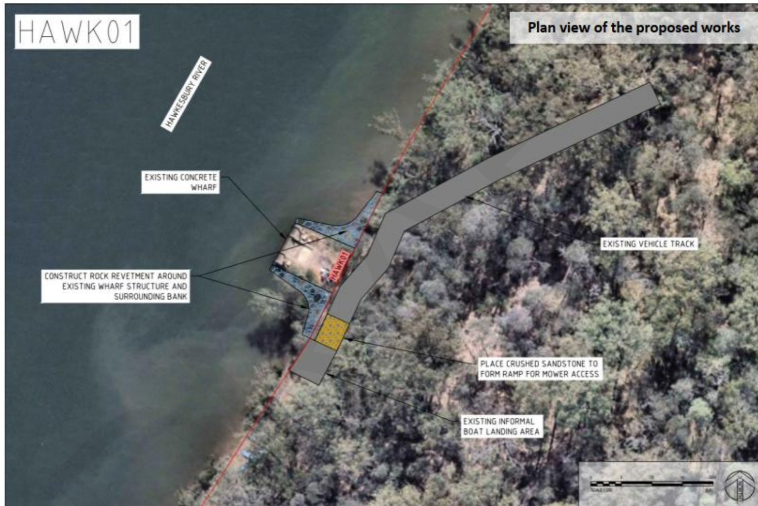
Figure C-26 Concept Design for Action S6.NPW.F at Gentlemans Halt. Source and further reference: (Alluvium, 2025)
