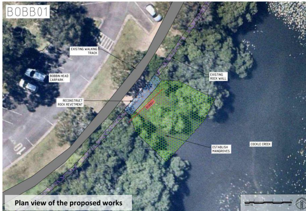
Figure C-30 Concept Design for Action S6.NPW.E at Bobbin Head (grouted rock wall section). Source and further reference: (Alluvium, 2025)
