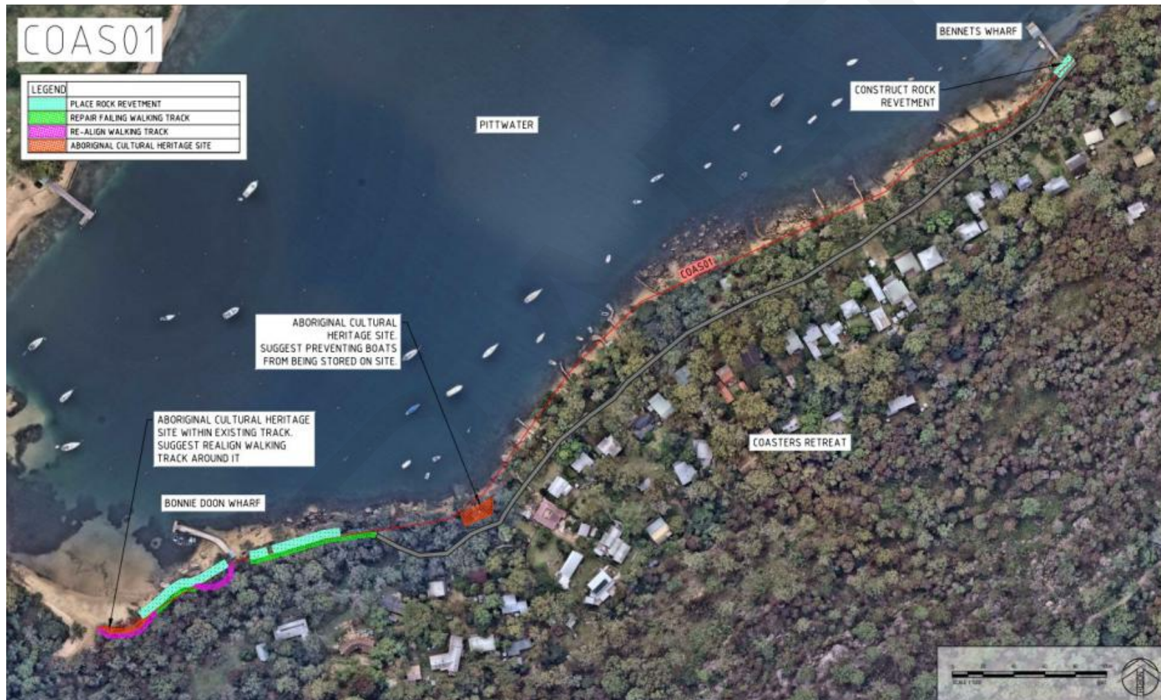
Figure C-18 Concept Design for Action S6.NPW.F at Coasters Retreat. Source and further reference: (Alluvium, 2025)
