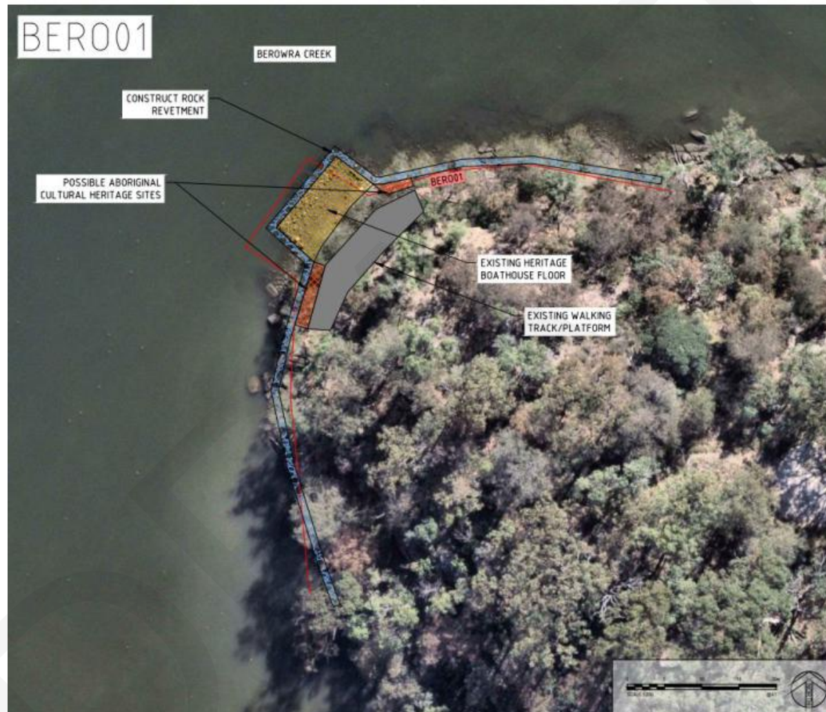
Figure C-22 Concept Design for Action S6.NPW.F at Berowra Creek. Source and further reference: (Alluvium, 2025)
